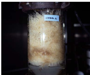
Figure 5. A 2.5-L ebb-and-flow bioreactor (EFBR) during gas dwell time and growing 18-day-old hairy roots.
